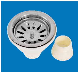
Regular 110mm round cap strainer with virgin PVC cup with SS plate, brass nut and reducer
